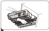
To raise the upper basket, just lift the upper basket at the center of each side until the basket locks into place in the upper position. It is not necessary to lift the adjuster handle.
