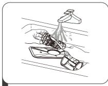
Larger food remnants can be cleaned by rinsing the filter under running water.
